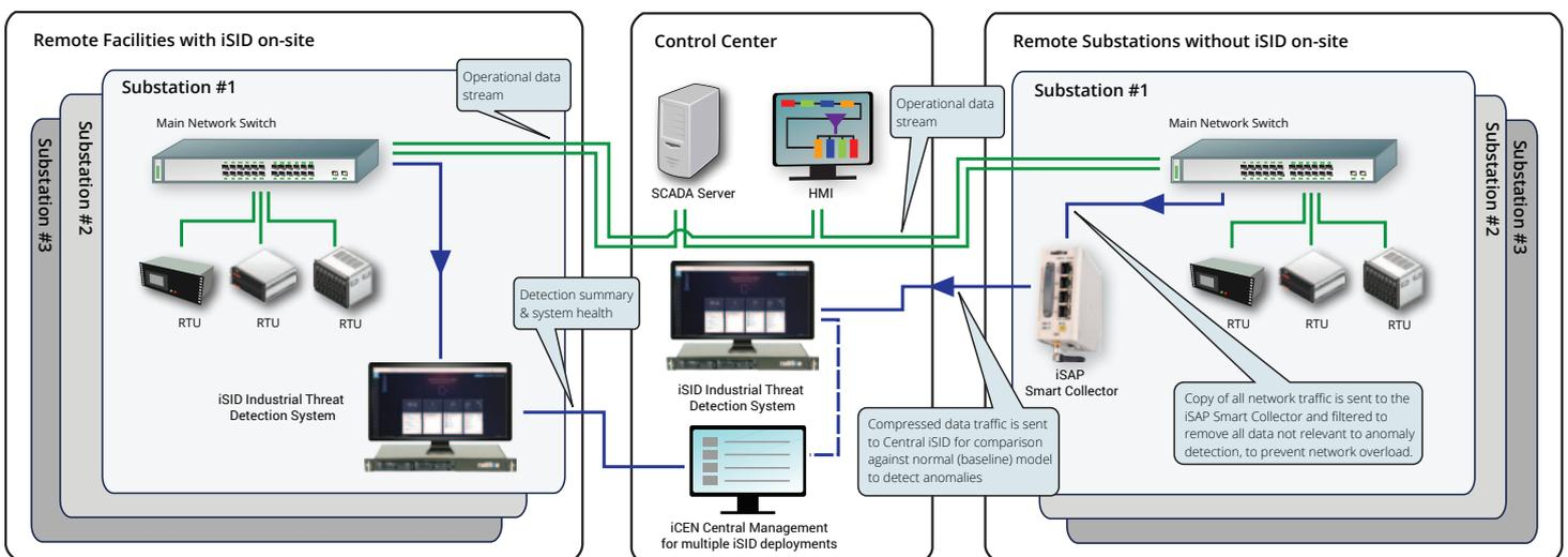
iSID deployment model, combining central deployment at control center and on-site deployment at remote sites (using iSAP Smart Probes)
